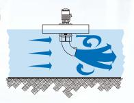
desirable. In such applications, the AquaDDM® with a directional flow assembly greatly reduces or eliminates short circuiting of the basin, eliminates deadspots and provides exceptional mixing of the basin contents.
