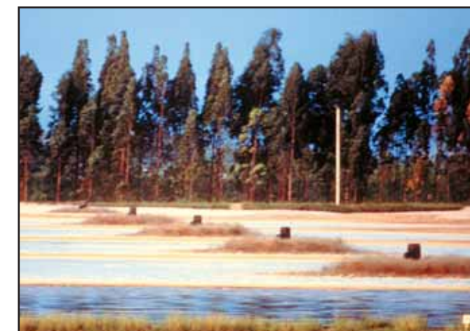
Aqua-Jet ® aerators increase the BOD removal efficiency at Smurfit Carton de Colombia.
