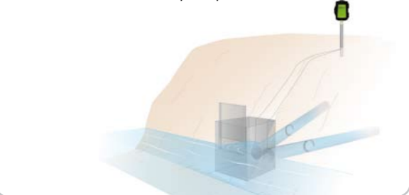
Lateral Diversion with Multiple Pipes
