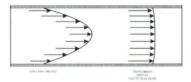
This means that the mixer approximates to a plug flow device. In a chemical reactor plug flow is very desirable as it would mean that each particle would be within the reactor for a known time. The Chemplant Static Mixer results in less byproduct formation.
