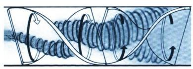
In laminar flow mixing occurs as a result of flow splitting and rotation. This builds up increasing number of layers of material each time fluid passes between two elements.
